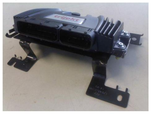
The original fastening clip is bent outward, so that the contact area increases for the control unit. Now it can be mounted on the bracket.
