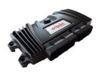
Fix the control unit at the original installation place. This is usually the chamber between engine and passenger cabin. Mount it in a slightly elevated position in order to protect it from intense moisture.
